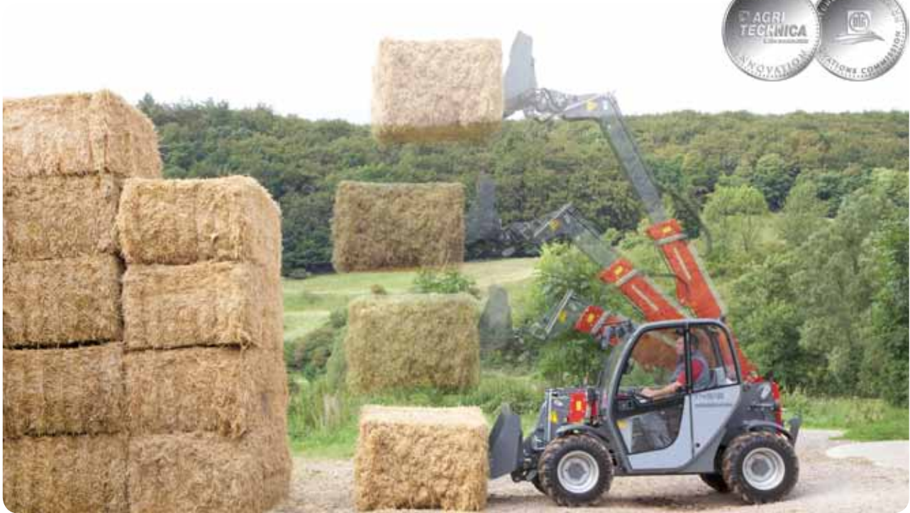
Weidemann Telehandler T4512. The new Vertical Lift System (VLS) enables operators to handle high payloads more smoothly. The key benefit of the new system is that it enables the telescopic arm to be lowered almost vertically, thus keeping the machine extremely stable. It was awarded a silver medal by a panel of experts at "Agritechnica", the world's leading exhibition for agricultural machinery.
